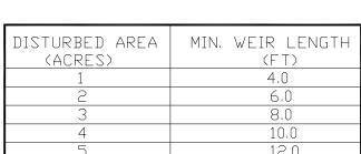
NOTE: THIS DESIGN IS FOR MAXIMUM DISTURBED AREAS OF FIVE (5) ACRES OR MAXIMUM TOTAL DRAINAGE AREA RUNDFF OF 30 CFS BASED ON A 10 YEAR STORM EVENT. FOR LARGER DISTURBANCES OR DRAINAGE AREAS, USE TEMPORARY SEDIMENT BASINS OR ROCK DAMS OR REDUCE DRAINAGE AREA BY USING MULTIPLE SEDIMENT TRAPS.
