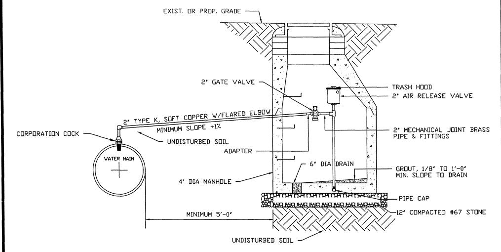
NOTE: 1. AIR RELEASE VALVE SHALL BE P-20 WITH VACUUM CHECK BY CRISPIN OR APPROVED EQUAL.
